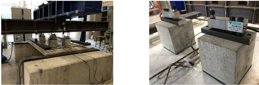
(a) (b) Figure 13 Experimental setup of predalles: (a) overview; (b) detail of load cells mounted on cubes
