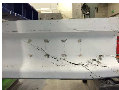
(a) shear failure Beam 4
